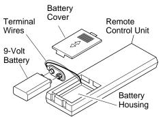
Figure 41 - Installing Battery in Hand-Held Remote Control Unit
